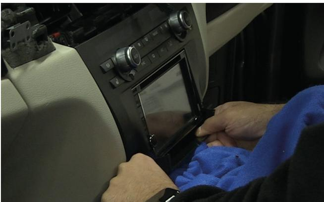
Take the bottom trim panel and slide it underneath the new stereo using the clip locators as guides to firmly clip it into place.
