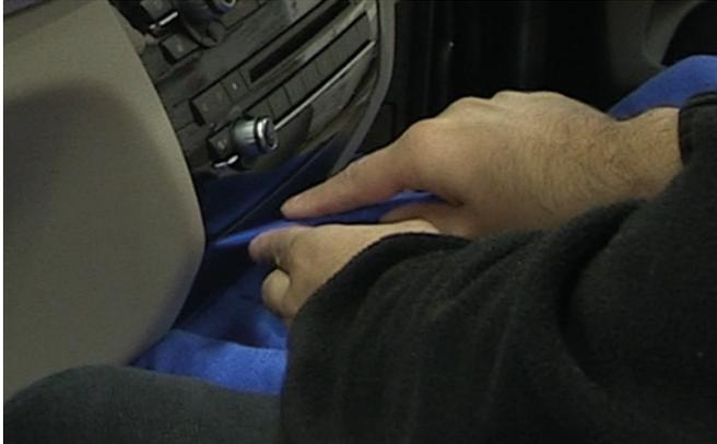
Begin by using a panel removal tool to remove the bottom trim panel.
