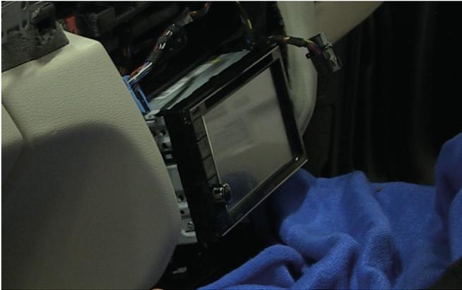
With the brackets affixed to the correct sides of the stereo, connect up the stereo and slot into place, screwing into place using the 4x pre-existing screws.
