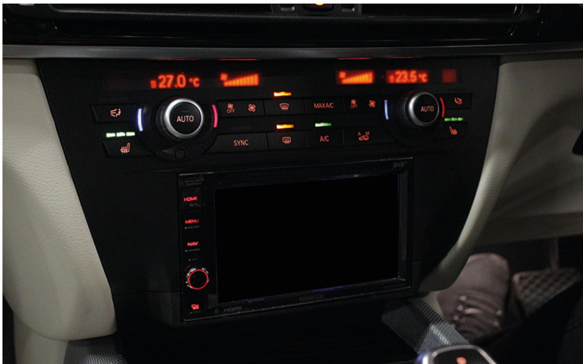
Reassemble the rest of the dashboard to complete the installation. When installed the vehicles original LED display will now be viewable alongside your new installed stereo.
