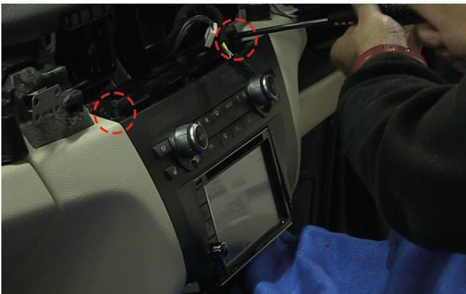
With the head unit fixed into position, place the new fascia over top, re-establishing the climate control connections. Once connected, use the 2x pre-existing screws to fix into place.
