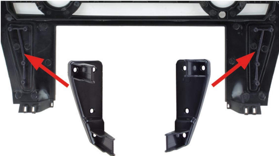
Take the 2x fascia locator brackets within the kit and line them up to the appropriate side of the fascia as indicated by the plastic grooves. Once lined up correctly, use the 8x self tapping screws to attach them to the back of the fascia.
