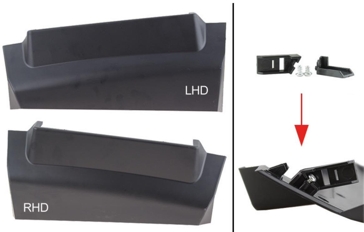
Select one of the bottom trim panels dependent on the orientation of the vehicle. Once selected, take the 2x locator clips found within the kit and attach them in the location seen here with the 2x screws provided. When fully attached, transplant the 2x OEM metal clips from the original bottom panel onto these locator clips.
