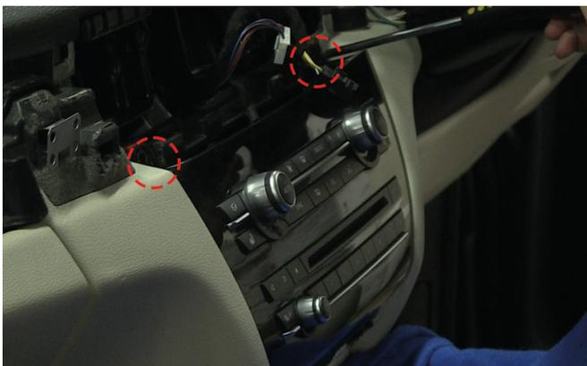
Once the air vent panel has been removed, it will reveal 2x screws that hold the main fascia panel in place. Remove both of these and disconnect all of the wiring.
